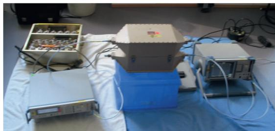
Figure 4: Measurement setup for determination of the shielding effectiveness
