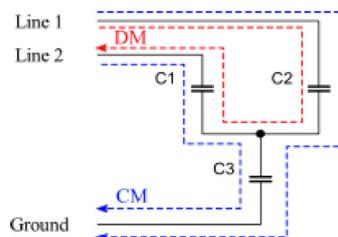
▲ **Figure 3:** Filtering: Common-mode and differential-mode
