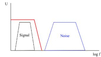
▲ **Figure 4:** Filtering out-of-band noise
