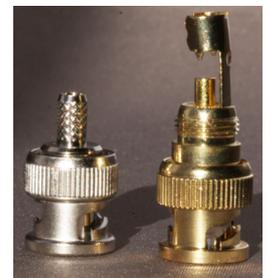
Figure 3: BNC Connectors, crimped version (left) and soldered (right).
